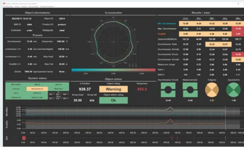
First screen display: Round profile with under-filling and a big defect, produced by a H/V stand
