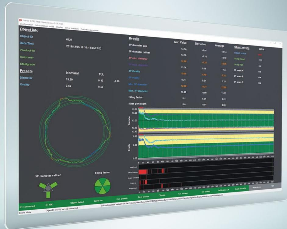
A typical screen for users: the green of the icons to the lower left shows that all measured values used to identify rolling faults are within tolerances.
