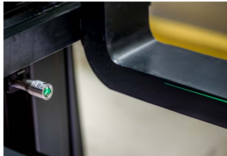
The XtrAlign HY positioning laser with a green laser diode is mounted between the fork arms on the fork carriage.
