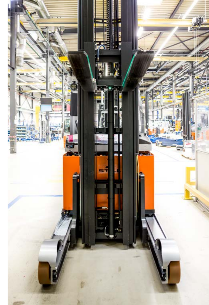
Line laser from LAP on the STILL FM-X 20 HD reach truck. Lifts loads of up to 2000 kilograms to heights of 13 meters at speeds of up to 0.50 m/s.
