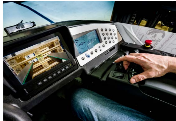
Full view of the situation: Drivers can see on a monitor when the exact target position has been reached.
