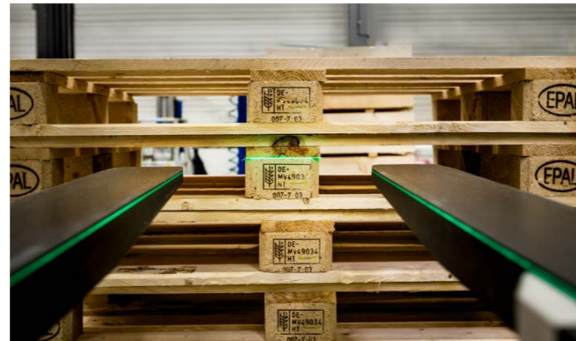
The clearly visible laser line precisely shows drivers at which height the fork arms need to move into the pallet's forklift pockets.
