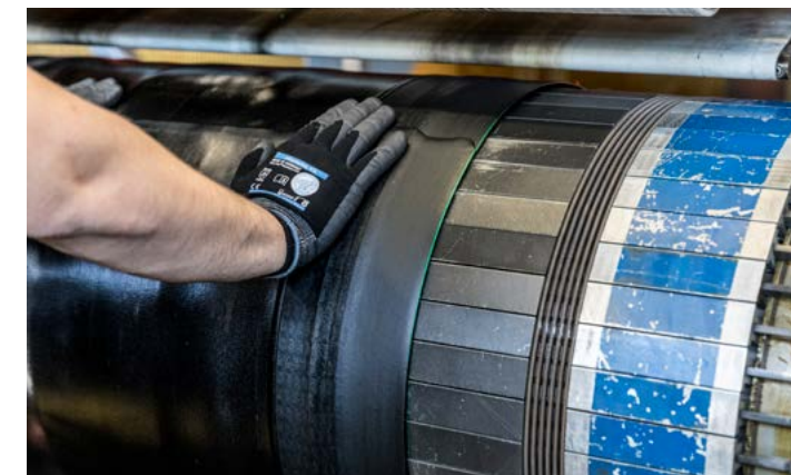
Changes by the minute: The precise positioning of each tire layer on the tire-building drum is checked using the laser lines. The green diodes of the latest SERVOLASER generation SLX provide even better visibility.
