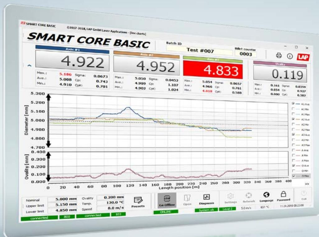
Standard view for a 3-axis round measurement with current measurement values and statistics by axis (top), line charts for diameter and ovality (middle), nominal and limit values (bottom left), and function buttons (bottom right)
