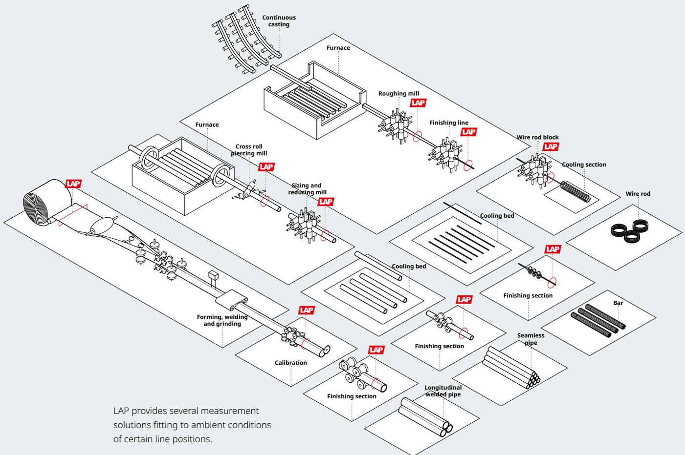
LAP provides several measurement solutions fitting to ambient conditions of certain line positions.
