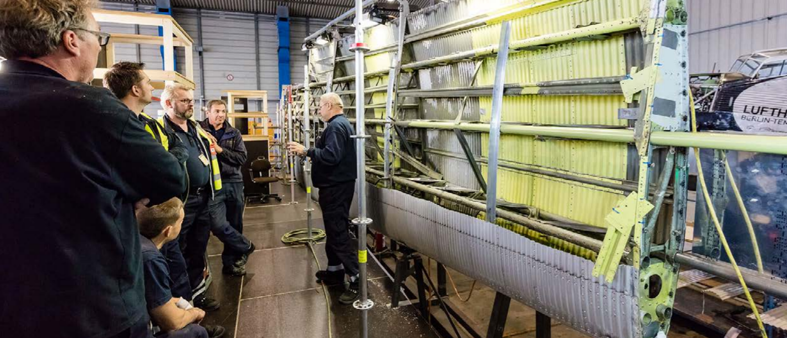
At the hangar on the Lufthansa base in Hamburg, the Ju received six new surface spars. Each spar is eleven meters in length and consists of six to eight segment tubes tapering towards the wing tips.
