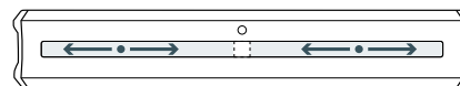
Symmetrical (laser modules move synchronously in relation to the middle of the rail)
