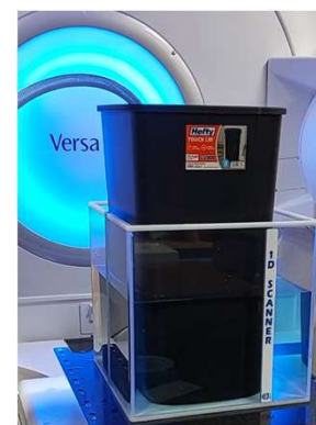
Figure 3: This image shows an H 2 O setup that can measure depths beyond 40 cm. With this setup, it is possible to accurately measure the response of EPID to transit beam dosimetry at greater depths.
